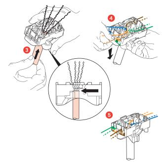
Spreading cables ensures that each pair is separated by the specified 13 mm.
