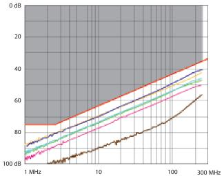
■ 9.2 Performance of permanent link with F/UTP cable Return loss
